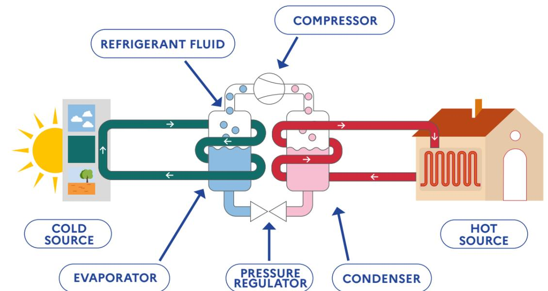
The working principle of a heat pump
